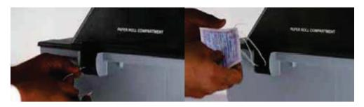
After installation of paper roll in the paper roll compartment of VVPAT, seal the latches of Paper Roll Compartment by passing a thread through holes provided on the latches using Address Tag showing the particulars of the election with the seal of the RO.
