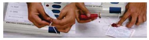
After unmasking candidate buttons, seal the upper cover of the BU by thread passed through holes on the top and bottom end at right side using address tags showing the particulars of the election with the seal of the RO.
