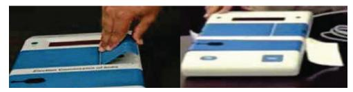
After Candidate set, seal cover of the Candidate Set Section and Battery Section of CU by passing a thread through hole provided on the respective side using address tags showing the particulars of the election with the seal of the RO.
