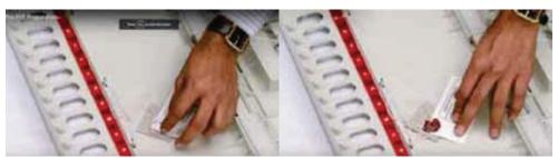
After firm fixation of the ballot paper under the Ballot Paper Screen on the upper side of top cover, seal the screen from inside, by passing the thread through two holes, at the back of the ballot paper screen, using address tag showing the particulars of election with seal of the RO.
