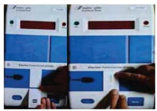
After sealing inner door of Result Section of CU with Special Tag, close the outer door of the Result Section ensuring that loose ends of the Green Paper Seal protrude out from both the sides of the closed outer door. Then the Presiding Officer shall seal the outer door by passing a thread through hole provided on the left side using Address Tag showing the particulars of the election with the seal of the Presiding Officer.
