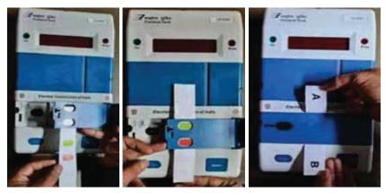
Fixing of Green Paper Seal and closing of inner compartment
